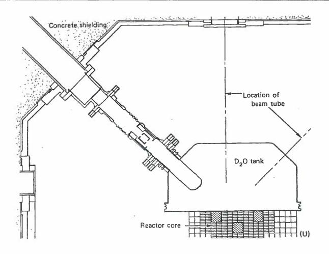
Fig. 1. Plan of neutron radiography facility at the Nuclear Research Center, Grenoble, France, showing a heavy water tank fitted to the Melusine reactor. (Redrawn from Ref. 1.)
